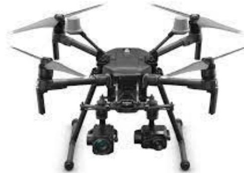
**Manufacturer Description:** UAS that has a color and infrared camera as well as audible speaker and light. Capable of video recording and weighs 899 grams, approx. 30 minutes of flight time. This is a remotely operated battery-powered aircraft designed to be operated within sight of the operator or a spotter. Each aircraft is equipped with a camera capable of relaying a real-time image back to the operator.
