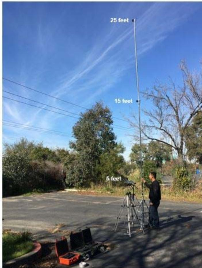
The results of the short-term ambient noise survey indicated that traffic noise exposure at the elevated floor locations was 3-5 dB higher than the measured ground-floor conditions during the same time period. As a result, a +3 dB offset would be warranted in the prediction of future traffic noise exposure at proposed 2<sup>nd</sup> floor locations, while a +5 dB offset would be warranted for the proposed 3<sup>rd</sup> and 4<sup>th</sup> floor locations.
