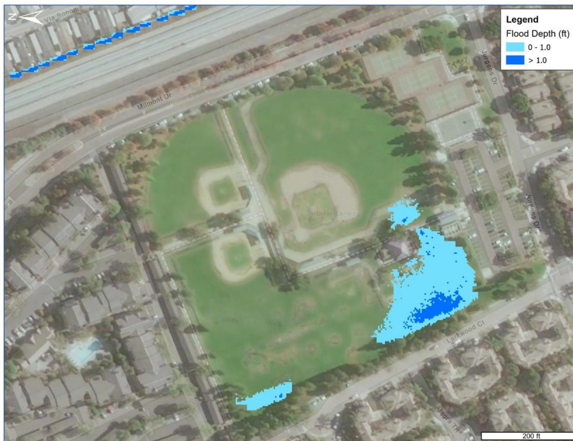
Figure 4-2: 10-year Ponding Adjacent to Jurgens Pump Station
