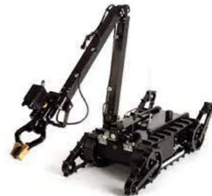
**Manufacturer Description:** The Mini Caliber is a lightweight, modular portable robot designed for rapid deployment, it is simple to operate and quick to deploy for searching rooms, hallways, stairwells, and confined spaces. It also includes an extendible rotating claw arm that simplifies opening door handles, providing protection and safety to their operators.
